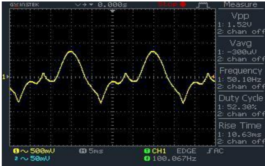
Figure (4-13) The wave form of the fault in the resistance (R12).
