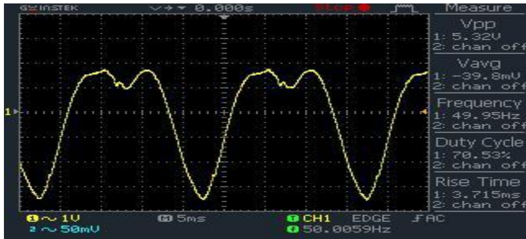
Figure (4-6) The wave form of the fault in resistance (R9)
